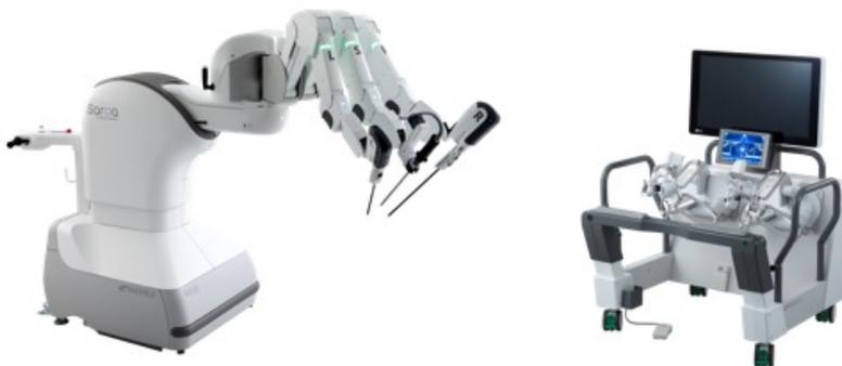
Figure 1. Saroa uses a standard flat-panel display rather than an immersive monitor, facilitating communication for the human surgical team
